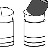
Insert the HI-C carbon filter into the funnel and hold it straight
